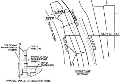
TYPICAL WALL CROSS SECTION, **ELEVATIONS SHOWN ON PLAN**
